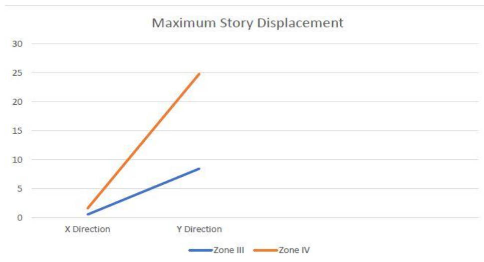
Fig.5 Maximum Story Displacement in Zone III and IV
